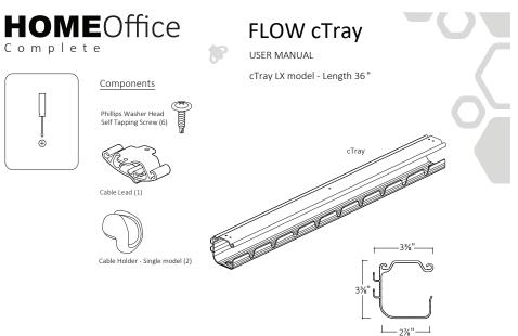
STEP 1: Attach cTray to underside of work surface.
