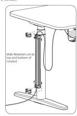
STEP 3.Insert the retainers onto the top and bottom of the conduit. The circular cut-out area on each retainer can face either direction.
