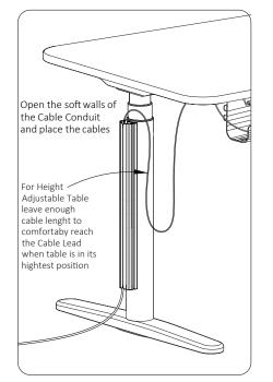
**STEP 3.** Place cable into the Conduit by pushing them down through the center of the Conduit.
