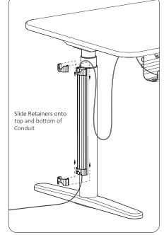
**STEP 4.** -Insert the retainers onto the top and bottom of the Conduit. -The circular cut-out area on each retainer can face either direction.
