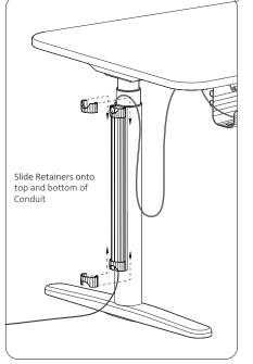
**STEP 4.** -Insert the retainers onto the top and bottom of the Conduit.
