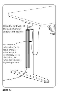
Place cable into the Conduit by pushing them down through the center of the Conduit.
