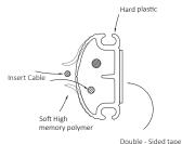
**WARNING**: When installing and using the product, act with care not to over bend to prevent breakage.
